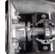
End bearing with shaft sealing group
