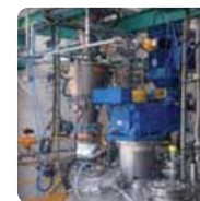
Implementation in harsh environments: loading of reactors in hazardous areas: protection of the filter against emanation of vapors, gas and dust area ATEX certification
