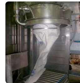
Hygienic conditioning of milk powder
