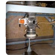
Rotary valve for product dosing
