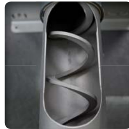
▶ Screw feeder for a high-accuracy dosing
