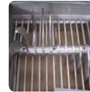
Integrated lump breaker enables the machine to handle powders with lumps. The blades ensure the passage of the lumps through a calibrated screen.
