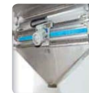
Vibrating chute allows to channel the material flow for introduction into the process upstream
