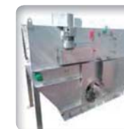
Extended body allows to process sacks with a maximum length up to 1 200 mm
