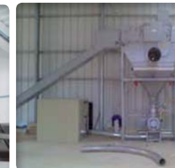
▶ Deconditioning of cement with pneumatic conveying
