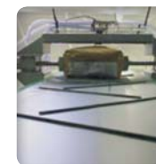
Pre-crushing of the bags during bags with lumps passage. The passage of the bag in front of the detect sensor starts the crushing action
