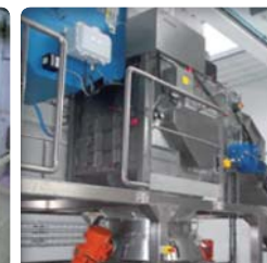
▶ Reactor feeding through a sifter
