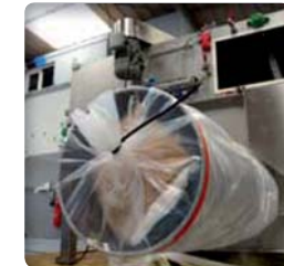
Screw compactor to compact and discharge bags into a plastic sheath to secure the outlet of the compactor
