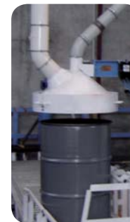
Puyès ring ensures the fine particles suction
