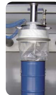
Inflatable seal provides a completely sealed filling
