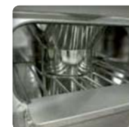
➤ Mirror-polished finishes to improve material flow and hygiene. Particularly suitable for the pharmaceutical industry
