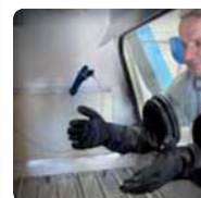
➤ Glove box for handling material in a closed and contained area: glass and gloves
