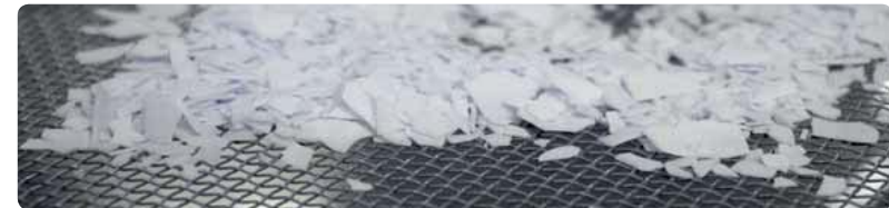
Integrated sieve: protection against foreign bodies for a production without any impurities.
