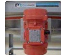
▶ Vibratory motor to improve the amplitude and intensity of the screen. These settings are adjustable depending on the flowability of the material and the mesh
