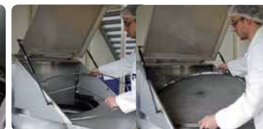
Easy access to the sifter including the screen mesh. Its design allows operators to clean and replace the screen mesh in seconds.
