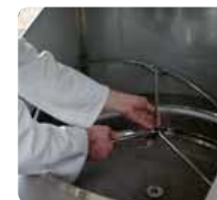
Easy access to the sifter including the screen mesh. Its design allows operators to clean and replace the screen mesh in seconds.
