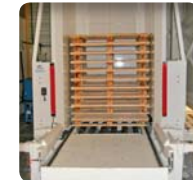
➤ Pallet unstacker for 15 of multi-format pallets
