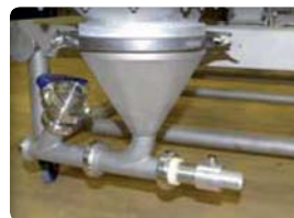
3 Venturi / Eductor Direct handling of the product create depression below the hopper Advantages • No rotating equipment • Ideal for light products on short to medium conveying lines • DN 50 to 150 mm.
