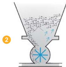
2 The material is directly blown into the blow-through rotary valve
