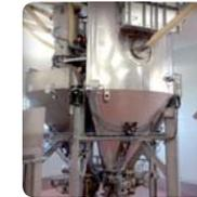
Net weighing hopper for customized filling
