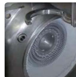
▶ Ultra fine grain size thanks to a very high rotation velocity: up to 6,000 rev./min.
