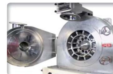
▶ Easy access to the grinding chamber thanks to a large door and possibility of tool changing: implanting of blades and calibrating cages
