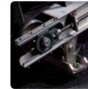
Belt tensing system
