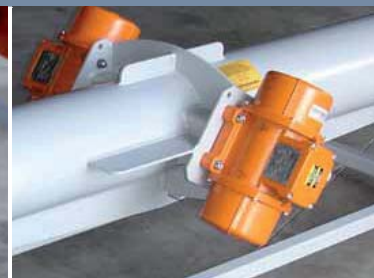
➤ Vibrating motor set on the tube with reinforcing barrel for power transmission
