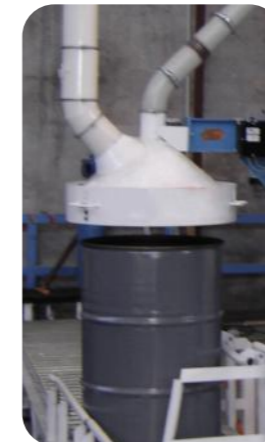
Pouyès ring ensures the fine particles suction
