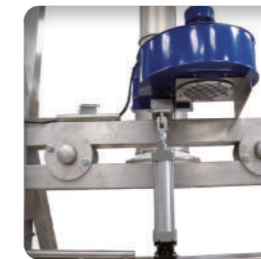
Fan and tension cylinder ensure big bag pre-forming and internal shaping
