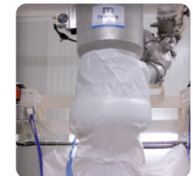
Inflatable seal to ensure dust containment for a clean workplace
