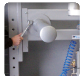
Adjustable fork height for an optimal filling of all types of big bags
