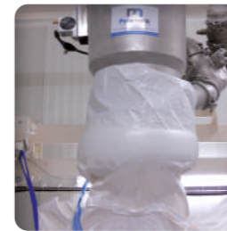
▶ Inflating seal to insure dust containment for a clean work area
