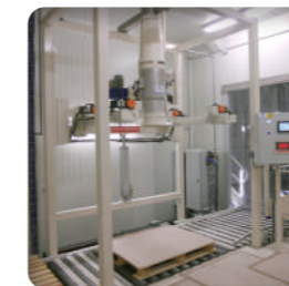
Dosing and weighing: automation and ergonomics of filling station
