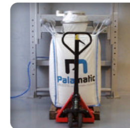
Big bag removal with pallet truck or lift truck
