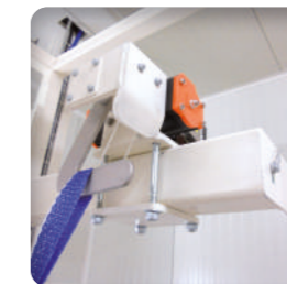
Automatic big bag release: process time optimization
