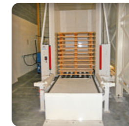
Pallet unloader can handle 15 multistyle pallets
