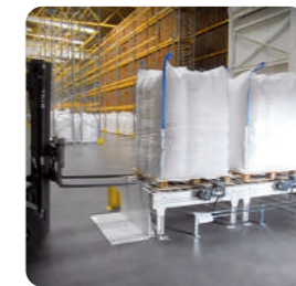
Big bag removal by lift truck
