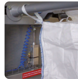
▶ Tension cylinder insures a perfect big bag filling and handling stability
