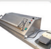
Welder for inner liner
