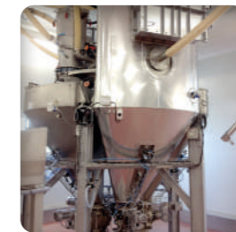
Net weighing hopper for customized filling
