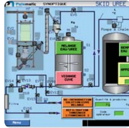
Control of a urea skid
