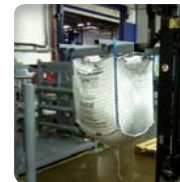
▶ Profiled push-buttons and control of dynamic strokes to avoid tearing the fabrics of the big bag
