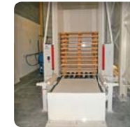
Pallet unloader can handle 15 multistyle pallets
