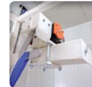
➤ Automatic big bag release: process time optimization
