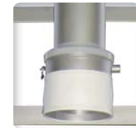
▶ Filling head with double envelope enables big bag air discharging through degassing line during the filling
