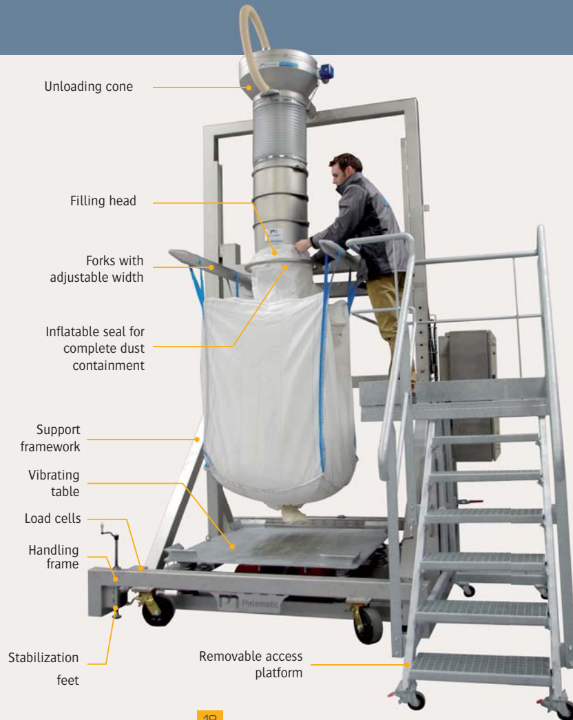
Load cells for dosing and commercial weighing
