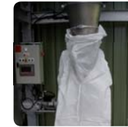
The fan inflates and shapes the big bag
