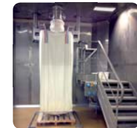
▶ Suspended structure facilitates floor cleaning
