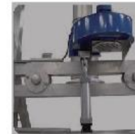
F Fan and tension cylinder provides bulk bag preforming and shaping
