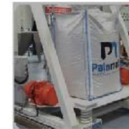
F Vibrating table provides densification for material volume reduction and stability of the bulk bag
