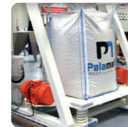
Vibrating table provides densification for material volume reduction and stability of the bulk bag
