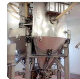
Net weighing hopper for customized filling
