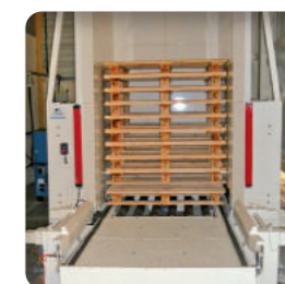
▶ Motorized conveyor for high production rates
