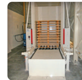
Pallet unloader can handle 15 multistyle pallets
