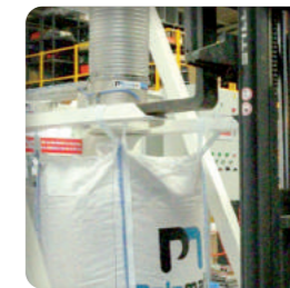
"U" shaped forks to remove bulk bag with straps
