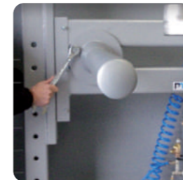
Adjustable fork height for an optimal filling of all types of big bags
