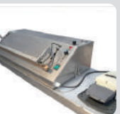
Welding for inner liner
