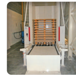
Pallet unloader can handle 15 multistyle pallets
