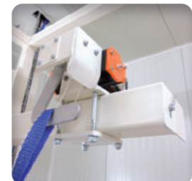
Automatic big bag release: process time optimization
