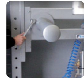
▶ Hooking forks width adjustment allows conditioning of all types of big bags
