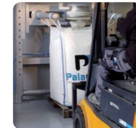
Big bag removal with forklift or pallet truck
