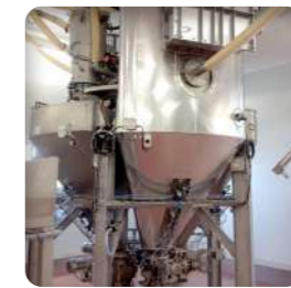
Net weighing hopper for customized filling
