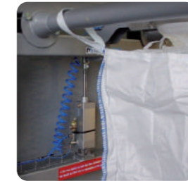
▶ Tension cylinder insures a perfect big bag filling and handling stability
