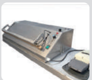
Welding for inner liner
