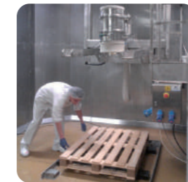
Hygienic design: the low ground coverage facilitates the cleaning process
