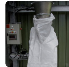
The fan inflates and shapes the big bag
