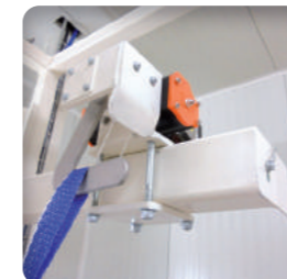
Automatic big bag release: process time optimization
