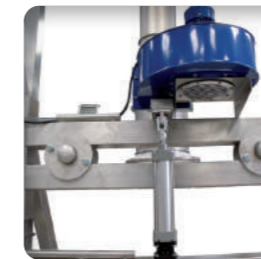
Fan and tension cylinder provides bulk bag preforming and shaping
