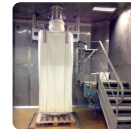
▶ Suspended structure facilitates floor cleaning
