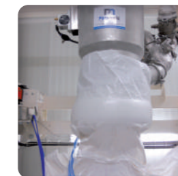
▶ Inflatable seal to ensure dust containment for a clean workplace
