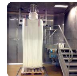
▶ Suspended structure facilitates floor cleaning
