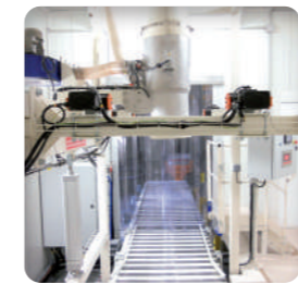
Motorized conveyor for high production rates
