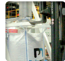
"U" shaped forks to remove bulk bag with straps
