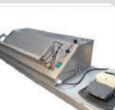
Welder for inner liner
