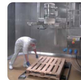
Hygienic design: the low ground coverage facilitates the cleaning process
