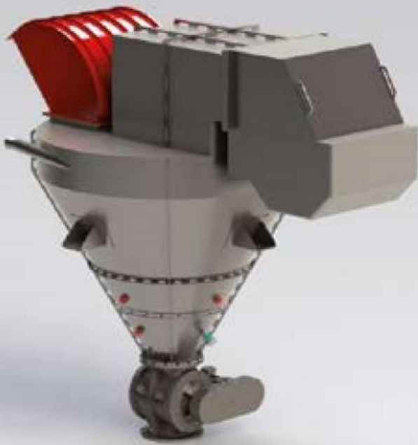
SolidWorks software representation of Atex cyclofilter, 30t./h.
