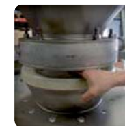
Dust cap seal to ensure the tightness of the connexion
