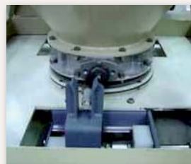
The opening of the valve can be performed automatically
