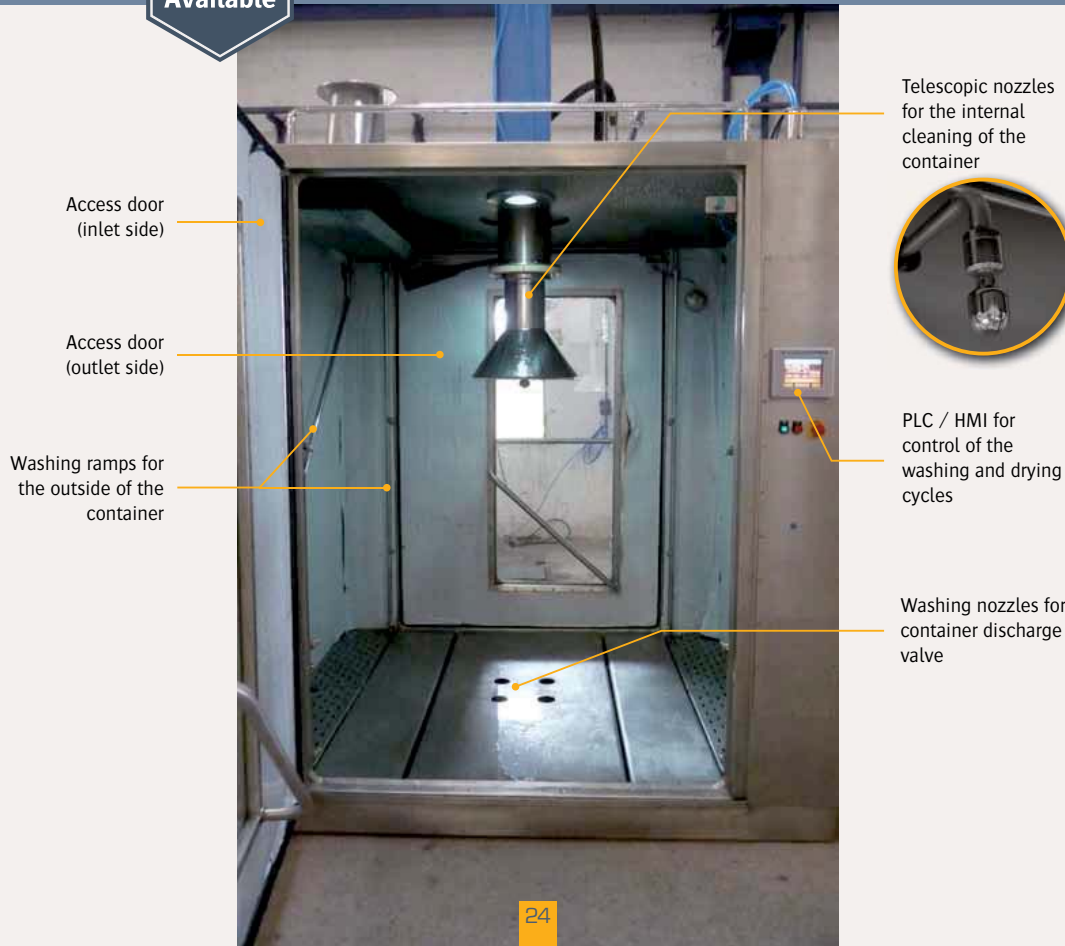
▶ Glass door with inflatable seals to monitor the washing process and ensure optimum sealing
