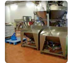
Open container for sack discharging
