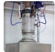
Sealing with inflatable seal to avoid any dust emanation and product loss
