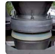
Dust cap seal to ensure containment and to allow high flow rates
