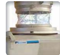
Fake lid with inflatable seal for total containment
