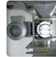
▶ ATEX version to resist to explosions and flame flow
