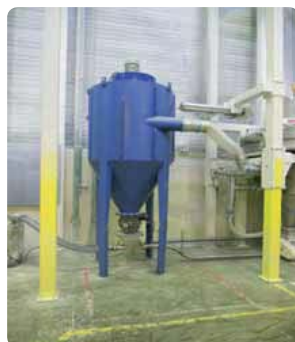
▶ Application under filter to insure the sealing and evacuation of fine particles
