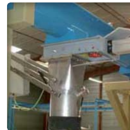
Cut off valve
