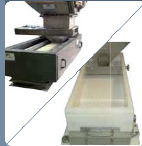
Belt / Vibrating Feeder
