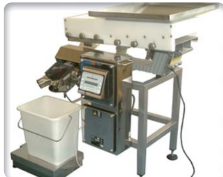
▶ Vibrating feeder with integrated metal detection for capsules
