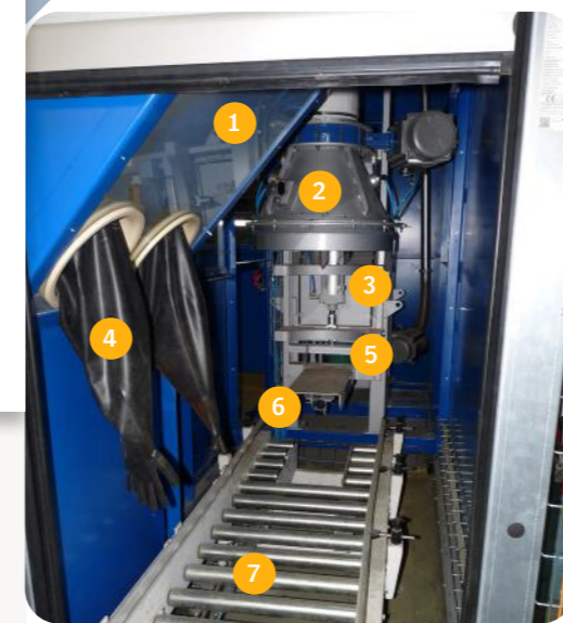
1. Containment enclosure - 2. Flow aid vibrator - 3. Containment cylinder - 4. Gloves for drum opening - 5. Tipping cradle - 6. Drum vibrator - 7. Motorized roller conveyor - 8. Butterfly Valve - 9. Inflatable Seal Connection - 10. Motorized group - 11. Butterfly valve for isolation of collection hopper - 12. Hopper - 13. Control panel - 14. Roller
