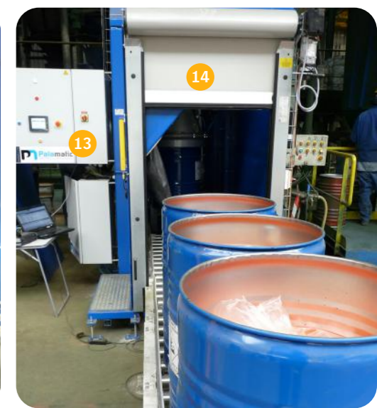
1. Containment enclosure - 2. Flow aid vibrator - 3. Containment cylinder - 4. Gloves for drum opening - 5. Tipping cradle - 6. Drum vibrator - 7. Motorized roller conveyor - 8. Butterfly Valve - 9. Inflatable Seal Connection - 10. Motorized group - 11. Butterfly valve for isolation of collection hopper - 12. Hopper - 13. Control panel - 14. Roller
