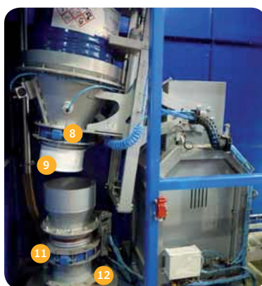
1. Containment enclosure - 2. Flow aid vibrator - 3. Containment cylinder - 4. Gloves for drum opening - 5. Tipping cradle - 6. Bottom drum vibrator - 7. Motorized drum preparation conveyor - 8. Dump valve - 9. Connection inflatable seal - 10. Motorized switching group - 11. Isolation valve of the collecting hopper - 12. Collecting hopper - 13. Control pannel - 14. Cabin with sectional door
