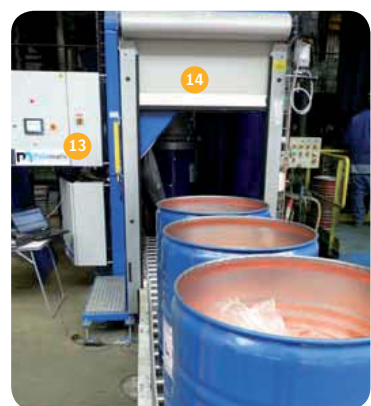
1. Containment enclosure - 2. Flow aid vibrator - 3. Containment cylinder - 4. Gloves for drum opening - 5. Tipping cradle - 6. Bottom drum vibrator - 7. Motorized drum preparation conveyor - 8. Dump valve - 9. Connection inflatable seal - 10. Motorized switching group - 11. Isolation valve of the collecting hopper - 12. Collecting hopper - 13. Control pannel - 14. Cabin with sectional door
