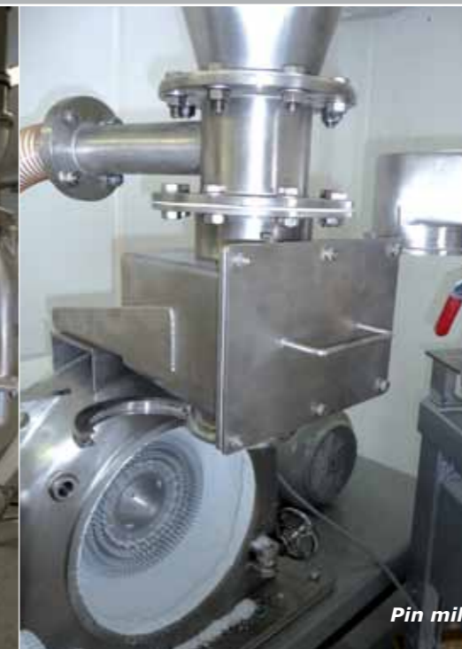
Atex mill with air vent
