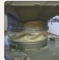
Flexible fitting on vibrating sifter
