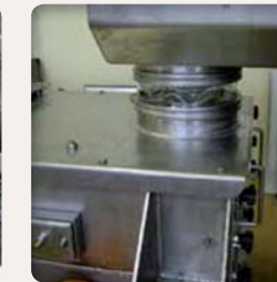
Connection between screw conveyor and sifter
