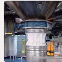
Fitting below butterfly valve with vacuum resistance
