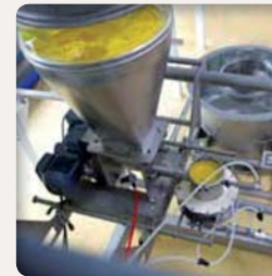
Feeding of large diameter dosing unit
