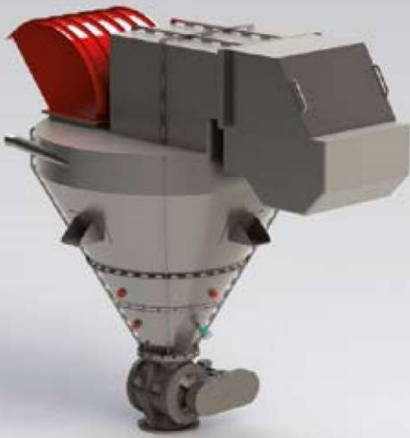
SolidWorks software representation of Atex cyclofilter for starch powder
