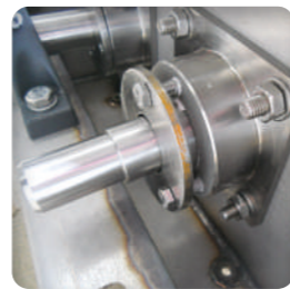
Shaft passage sealing
