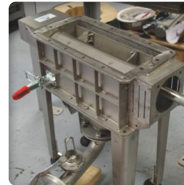
▶ Granulator feeding the vacuum pneumatic conveying system
