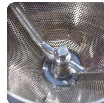
▶ Conical lump breaker for veterinary products
