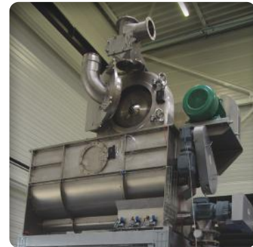
▶ Icing sugar grinding with mixing tank
