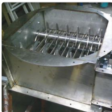
▶ Lump breaker with knives integrated into a big bag dumping station for wax tablets processing
