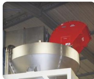
2 The explosion vent allows the evacuation of the explosion pressure
