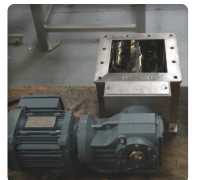
▶ Lump breaker EC35 for sugar application
