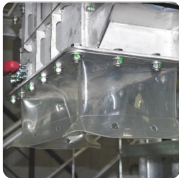
▶ Granulator integrated in a dump station
