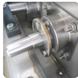
Shaft passage sealing
