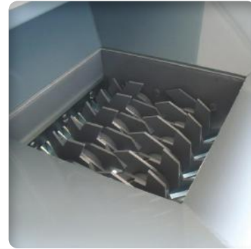
▶ Lump breaker for road salt
