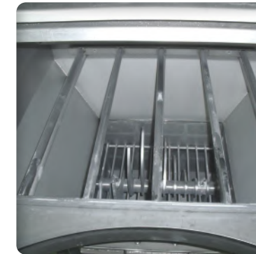
▶ Lump breaker integrated on a bag dump station of resin flakes
