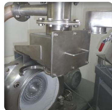
▶ Magnetic bars in food grinding process
