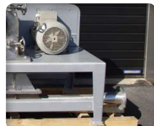
5 The venturi ensures the conveying of the micronized powder
