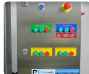
4 The control panel ensures management of doses and flow rate
