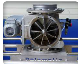
1 The rotary valve ensures the isolation of the volumes
