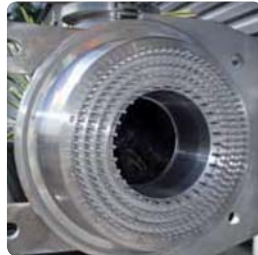
▶ Fix part of the grinding mill
