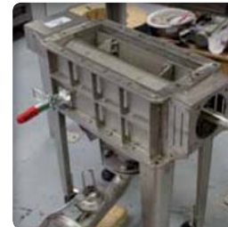
▶ Granulator feeding the vacuum pneumatic conveying system
