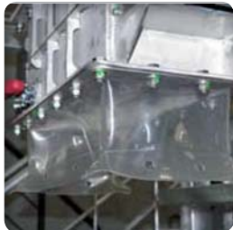
▶ Granulator integrated in a dump station
