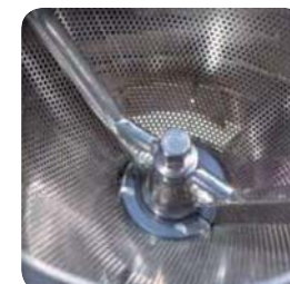
▶ Conical lump breaker for veterinary products
