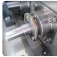
Shaft passage sealing
