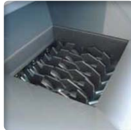
▶ Lump breaker for road salt
