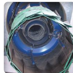
Dustproof skirt ensuring the suppression of dust raised during loading operations
