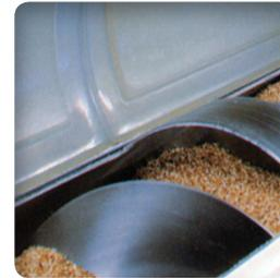
▶ **Minimum gap (flight clearance) between the tube and external screw flight (max. 5 mm.)**
