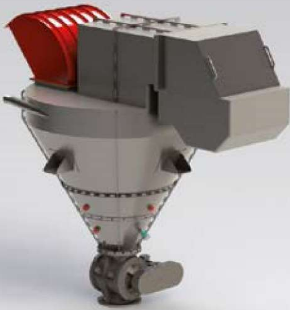
Solidworks software representation of conveying cyclofilter
