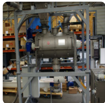
▶ Mixing skid the debacterization of seaweed powder (cosmetic application)
