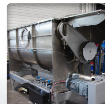
▶ Chain drive of the agitation device
