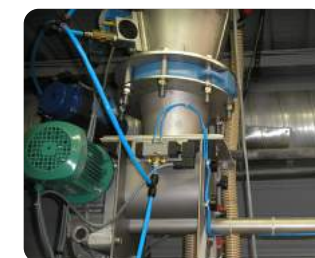
3 Dosing system for incorporation of lime
