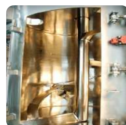
Polishing of welded components for hygienic finish
