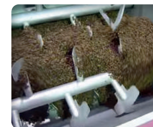
2 Double shaft mixer with blades
