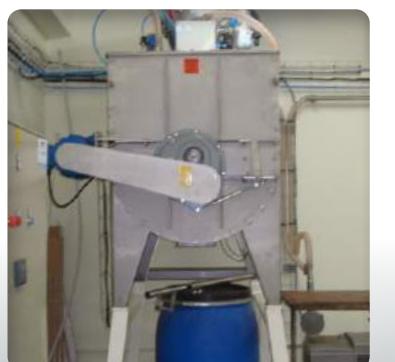
► Mixer with detached engine
