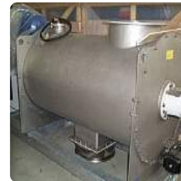
► Stainless steel cylindrical mixer
