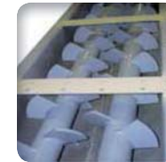
▶ Self-cleaning rotors thanks to overlapping blades
