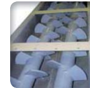
▶ Self-cleaning rotors thanks to overlapping blades
