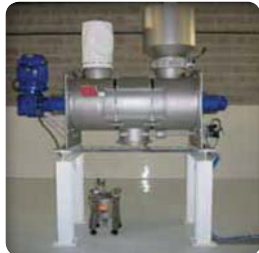
▶ Laboratory mixing skid with incorporation of liquid
