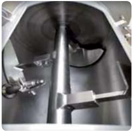
▶ Inside view of the mixer with blades and chopper made of stainless steel
