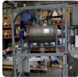
▶ Mixing skid for the debacterization of seaweed powder (cosmetic application)
