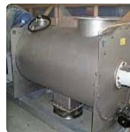
▶ Stainless steel cylindrical mixer
