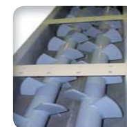
▶ Self-cleaning rotors thanks to overlapping blades
