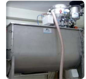
► Loading of the trough mixer with pneumatic conveying
