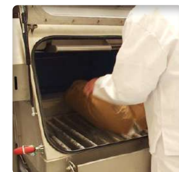
The operator folds and shakes the sack to release the material with minimal effort. The operator does not have to turn the bag over.
