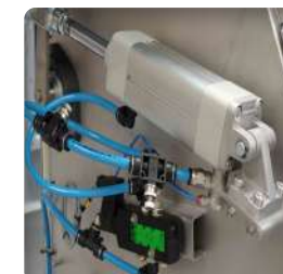
Pneumatic cutting cylinder with accumulator for optimal cutting
