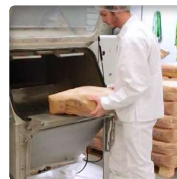
The operator places the sack on the safety grate and uses both hands to actuate the controls for the cutting blade.
