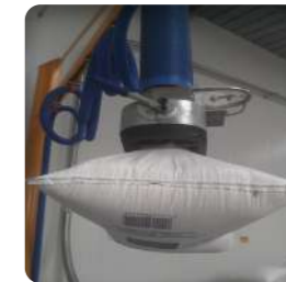
Hessian bags: vacuum spike gripper to lift sacks of grains
