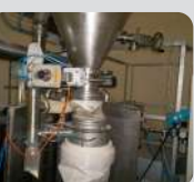
Sack unloading unit with dedusting panels
