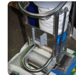
Vacuum sack lifter: fitted with a control handle equipped with a stay-put lever valve allowing a self-stabilization of the load at any height, without any adjustment. Ergonomic handle design, preventing wrist elongation
