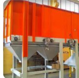
Vibrating chute to ease and control the flow of the material
