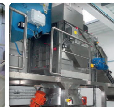
➤ Reactor feeding through a sifter
