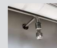
Nozzles/washing rotary heads (CIP)
