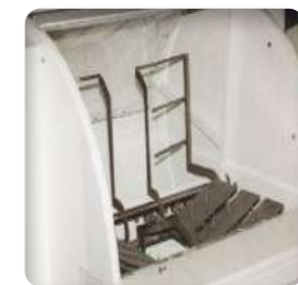
Ejection of empty bags into the compactor
