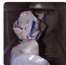
▶ Rotative drum: separation of powders and sacks
