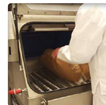
The operator folds and shakes the sack to release the material with minimal effort. The operator does not have to turn the bag over.
