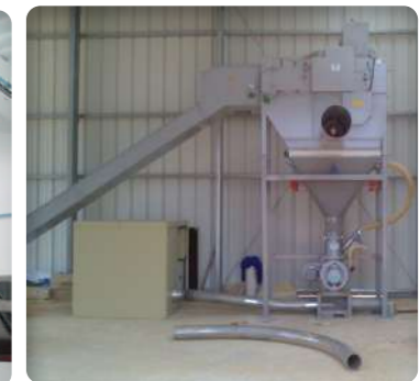
➤ Deconditioning of cement with pneumatic conveying
