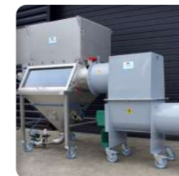
Handling wheels for mobility of the equipment (optional)
