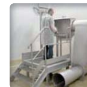
Ergonomic access for the operator: the height is appropriate and it is possible to integrate a platform
