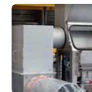
➤ Side discharge chute for the bag to maintain a clean working area and to eject the "dirty" emptied sack in a contained area
