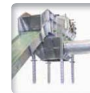
Support raiser for the machine to enable the operator to have access to the various doors of the machine
