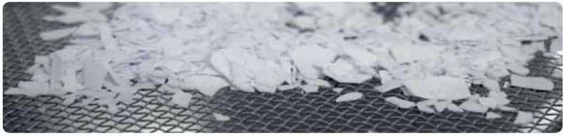
Integrated sieve: protection against foreign bodies for a production without any impurities.
