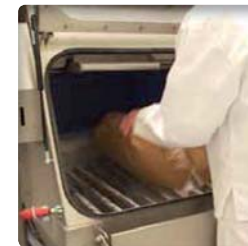
▶ Shaking of the sack without effort and without heavy lifting of the sack. The operator does not have to return the bag.
