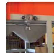
▶ Vibrating chute allows to channel the material flow for introduction into the process upstream
