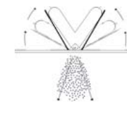
3. Shaking of the sack with articulated plates
