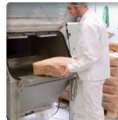
▶ The operator puts the sack down on the grate and actuates the control of cutting.
