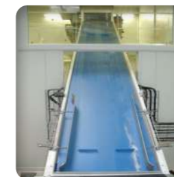
Belt conveyor , horizontal or inclined. It integrates detection cells to adjust the flow rate of the machine
