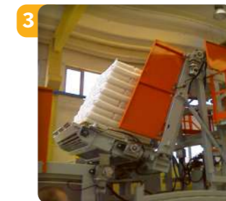
3 Tilting of the full pallet directly into the machine
