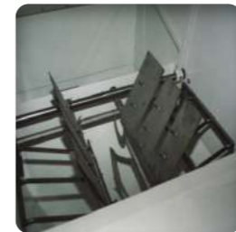
▶ Internal mobile parts of the machine ensuring the shaking and the ejection of the sacks
