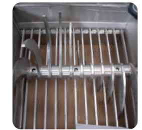
Integrated lump breaker enables the machine to handle powders with lumps. The blades ensure the passage of the lumps through a calibrated screen.
