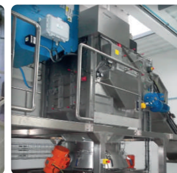
▶ Reactor feeding through a sifter
