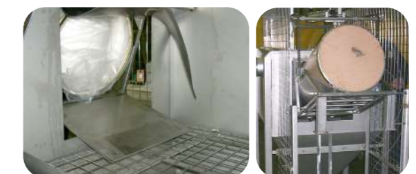
Lifting and positioning of the drum in the booth is performed by the elevator integrated on the booth
