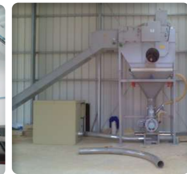
▶ Deconditioning of cement with pneumatic conveying
