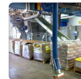
▶ Vacuum lifter to handle effortlessly sacks for an ergonomic working station (option)
