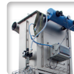
Dust collector ensuring healthy work environment
