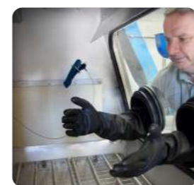
▶ Glove box for handling material in a closed and contained area: glass and gloves
