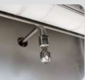
Nozzles/washing rotary heads (CIP)
