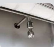
Rotative cleaning nozzles/heads - Clean In Place (CIP)
