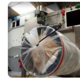
▶ Screw compactor for the evacuation of the emptied sacks and the reduction of dust emissions
