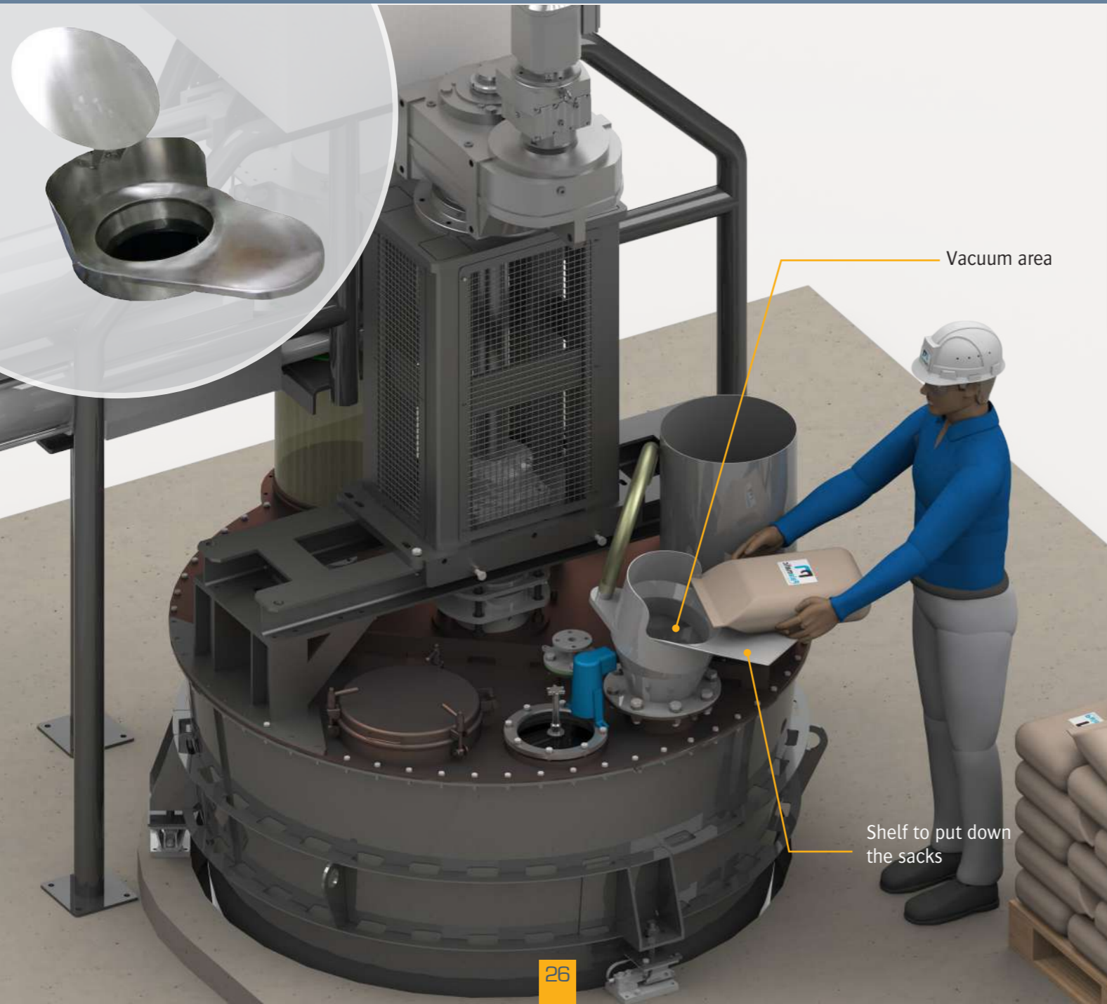
▶ Simplified ring for suction on the periphery of a vertical mixer vertical
