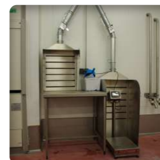
Suction booth with integrated scale
