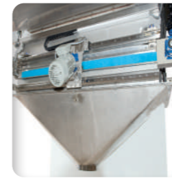
Vibrating spout for dosing and homogeneous separation of your bulk materials.
