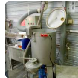
▶ Simplified ring for suction on the periphery of a vertical mixer vertical
