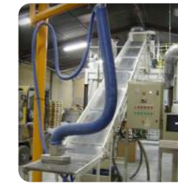
Vacuum lifter for sacks for effortless handling and improvement of the productivity
