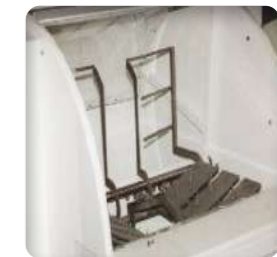
▶ Ejection of empty bags into the compactor
