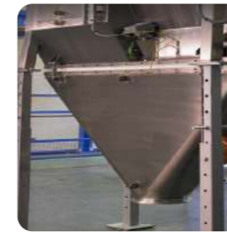
Stainless steel static chute for the transfer of the powders into the process
