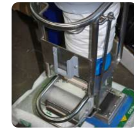
▶ Vacuum sack lifter: fitted with a control handle equipped with a stay-put lever valve allowing a self-stabilization of the load at any height, without any adjustment. Ergonomic handle design, preventing wrist elongation
